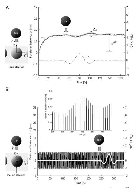
**Fig. 6.** The computed motions of (A) the free electron and (B) the bound electron, under the combined external electric  $\vec{E}$  and ionic  $\vec{F}^{ion}$  force. The dashed line represents the ionic force  $\vec{F}^{ion}$  and the solid line represents the position of the electron. The ion collides with (A) the free electron at t=50 fs and (B) bound electron at t=250 fs.
