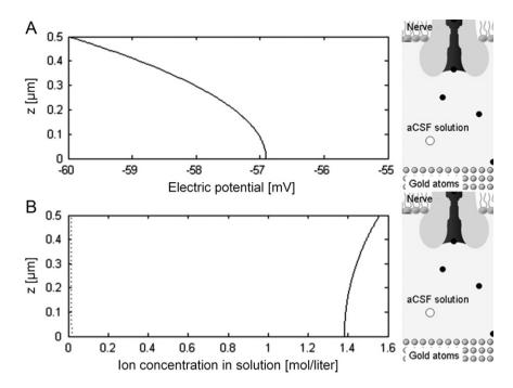
**Fig. 4.** The *z* directional (A) electrostatic potential and (B) ion density profiles at a fixed resting nerve's recorded extracellular potential  $u_m$  of -60 mV. The solid line is the counter ion density and the dashed line is the anion density.
