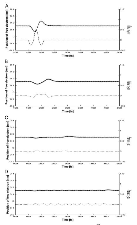
**Fig. 7.** The computed instantaneous motions of the free electron at various configurations of the ionic forces  $\vec{F}^{ion}$  produced from the superposition of 10 unit ionic forces  $F^{ion}_i$  with various time steps. The time intervals divided by collision duration  $\Delta t_{i_1}/\tau$  were (A) 0, (B) 0.071, (C) 0.212 and (D) 0.48. For details, see text.
