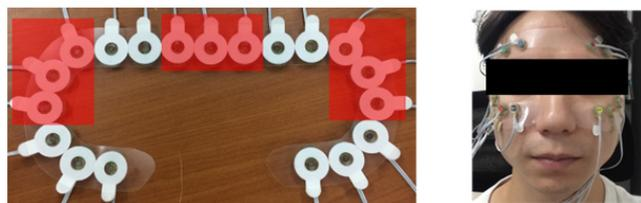
**FIGURE 1.** HMD pad for recording fEMGs and a user wearing an HMD pad with ten electrodes. Nine electrodes within the shaded rectangles were excluded in this study.
