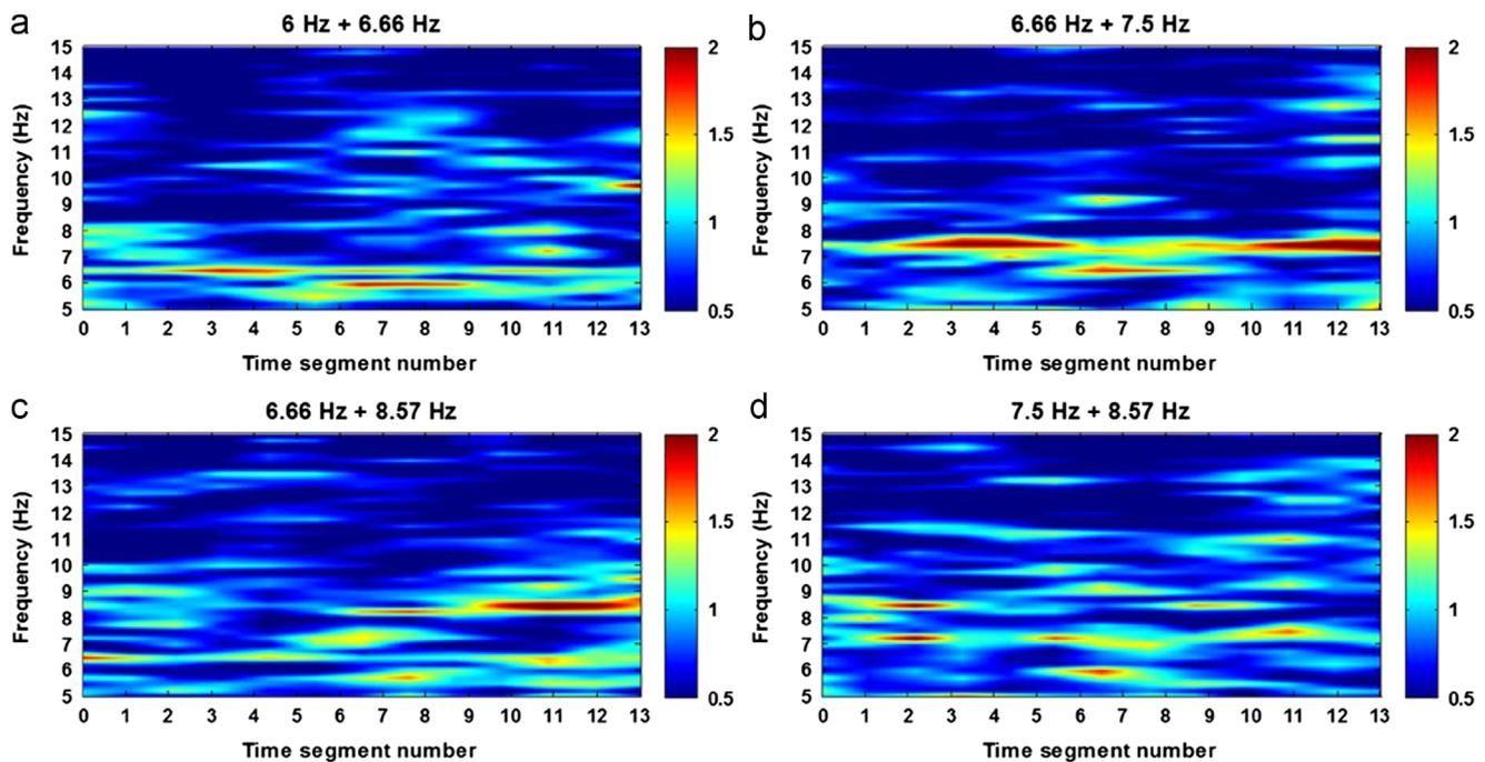
**Fig. 2** – Time–frequency pattern maps of a participant (P1) demonstrating time-varying amplitudes of two fundamental frequencies: (a) SSVEP responses when 6.66 Hz and 7.5 Hz were used as stimulating frequencies, (b) SSVEP responses when 6 Hz and 6.66 Hz were used as stimulating frequencies, (c) SSVEP responses when 6.66 Hz and 8.57 Hz were used as stimulating frequencies, and (d) SSVEP responses when 7.5 Hz and 8.57 Hz were used as stimulating frequencies. Units:  $\mu\text{V}^2$ .
