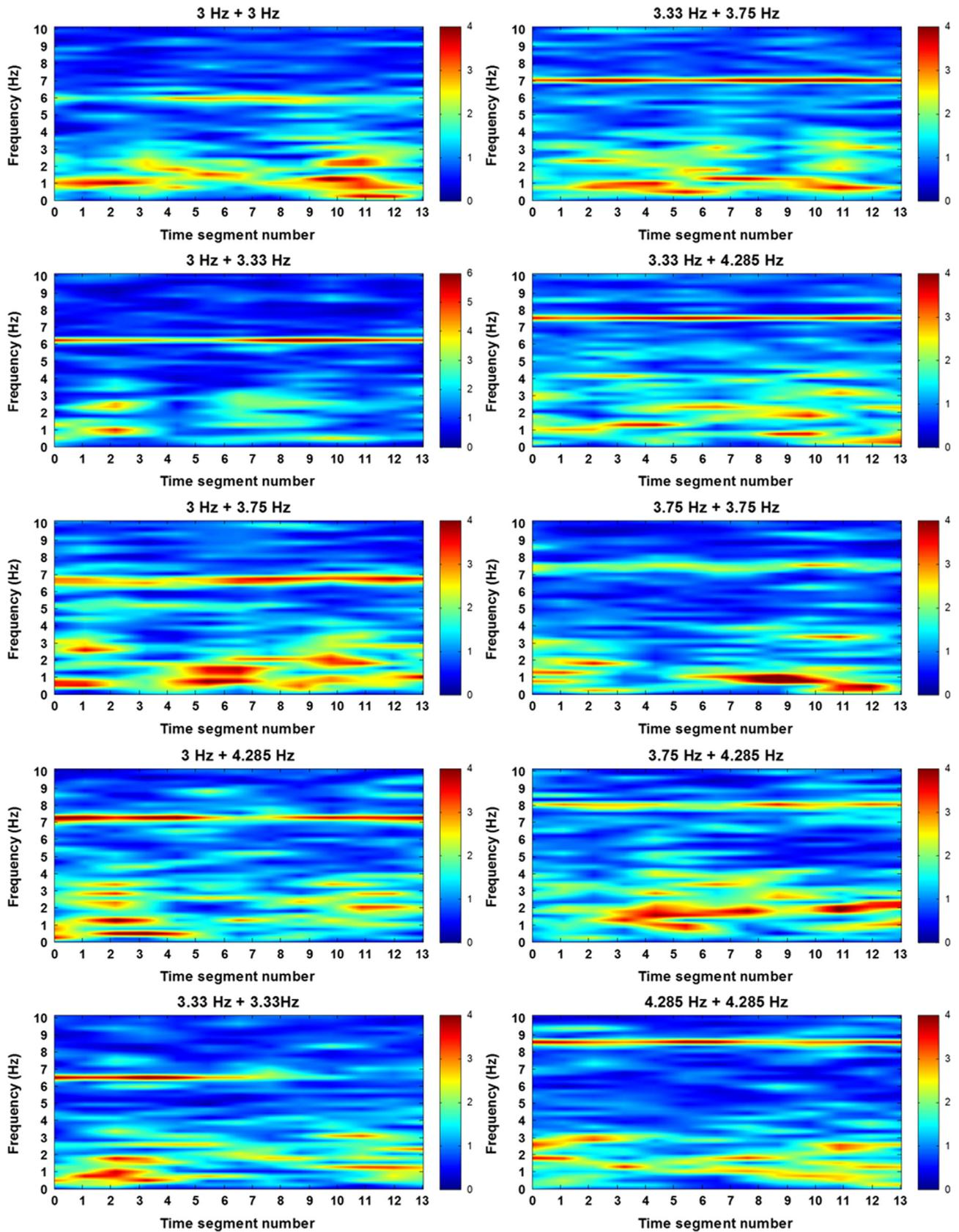
Fig. 4 – Time–frequency pattern maps of a participant (P1) acquired while he was staring at the ten different visual stimuli generated by combining four different frequencies (3 Hz, 3.33 Hz, 3.75 Hz, and 4.285 Hz). Units:  $\mu\text{V}^2$ .
