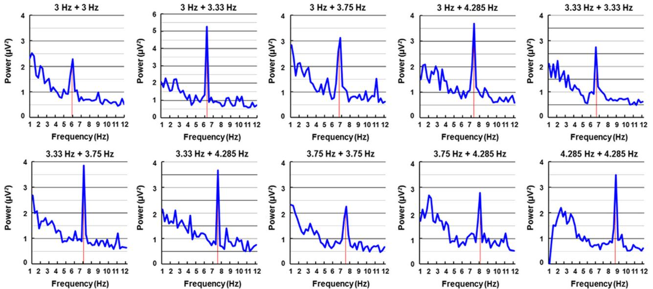
Fig. 5 – Spectral powers averaged over the 30-s epoch shown in Fig. 4. Four different frequencies (3, 3.33, 3.75, and 4.285 Hz) were used to generate ten visual stimuli. Distinct SSVEP peaks were observed at the sum of two fundamental frequencies for every stimulus. Note that the range of the y-axis for the 3 Hz+3.33 Hz result is from 0 to 6, while the others range from 0 to 4.
