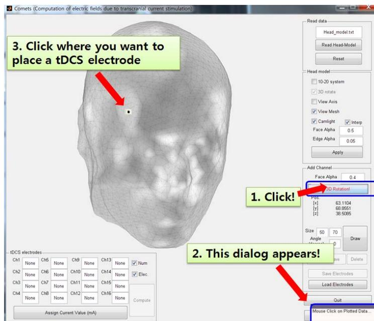
**Figure 6** The procedure for determining the position of the candidate electrode
